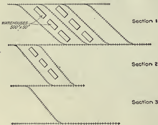
FIG. 1. SKETCH SHOWS TYPICAL LAYOUT OF WAREHOUSE SECTION OF ARMY INTERMEDIATE DEPOT
