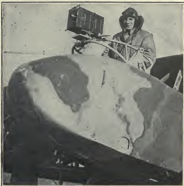
THE AIR CAMERA IS FLEXIBLY MOUNTED
