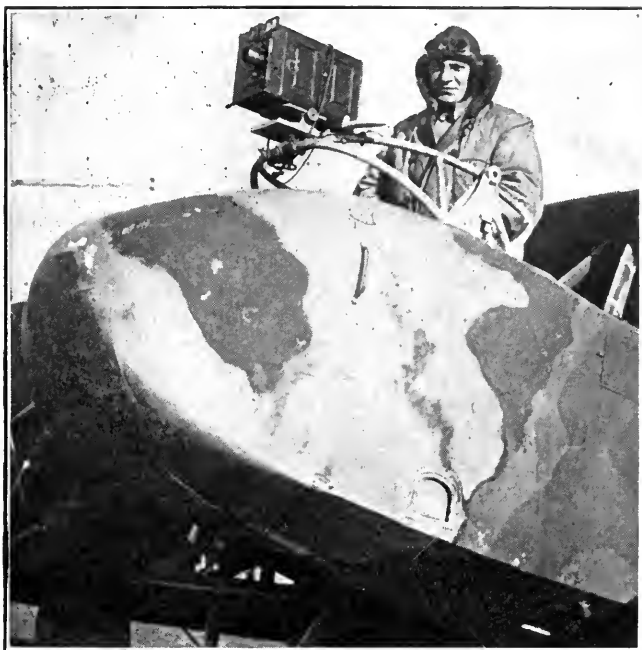
THE AIR CAMERA IS FLEXIBLY MOUNTED
