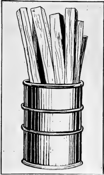
Showing bark and treatment of timber with Grade-One Creosote Oil.
