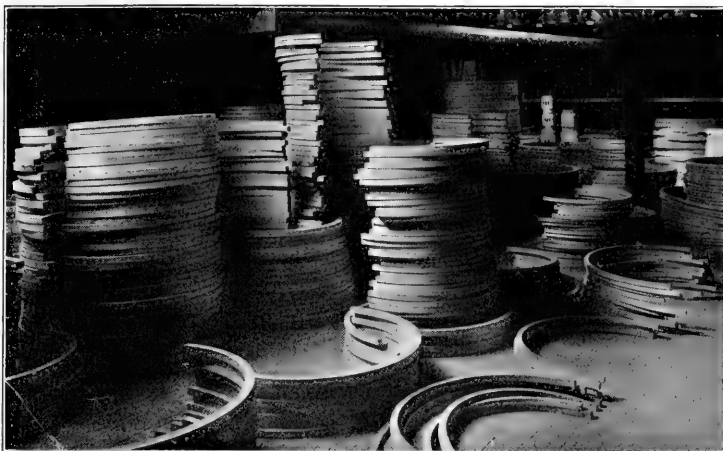
HICKORY USED FOR WHEEL RIMS
