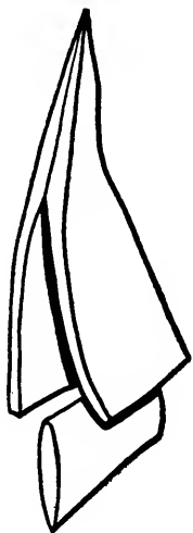
FIGURE 5. Construction of a spiked hatchet with two pieces of iron and a steel edge.
