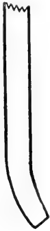
FIG. 6. Lower end of glass cannula for perfusing the ramus circumflexus in the living animal.
