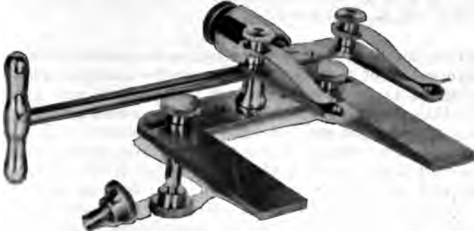
Fig. 2. New model of instrument, showing revised form of foot-plate, with sliding posts adjustable to clip-holes of any stage; an extra pair of these posts shown at the left. Key is in position. The clips may be inserted in all four corners of the elevated clip-plate, and thus turned backward or cross-wise.
