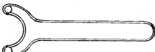
Pin-face, For Round Nuts Having Holes in their Face to Receive the two Wrench Pins
