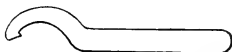
Hook Spanner, Milled out to suit Round Nuts Having Notches in the Periphery to Receive the Hook at the End of Spanner
