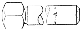
DIMENSIONS OF BLANKS FOR U. S. S. ROLLED THREAD SCREWS (REED & PRINCE MFG. CO.)
