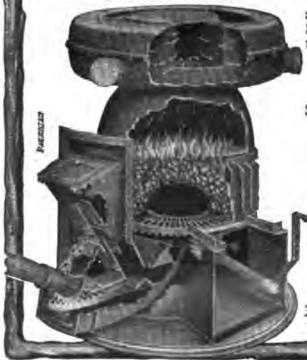
Illustration shows furnace, without casing, cut out, to show how coal is forced up under fire—which burns on top.
