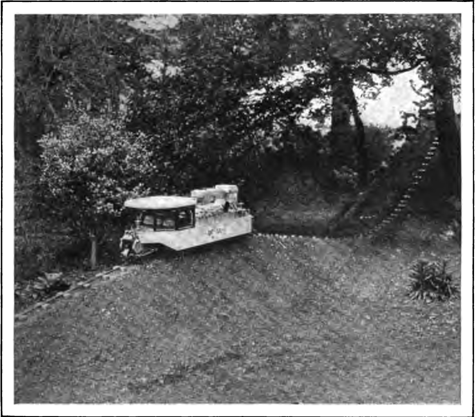
The rail may undulate up and down over rough ground
