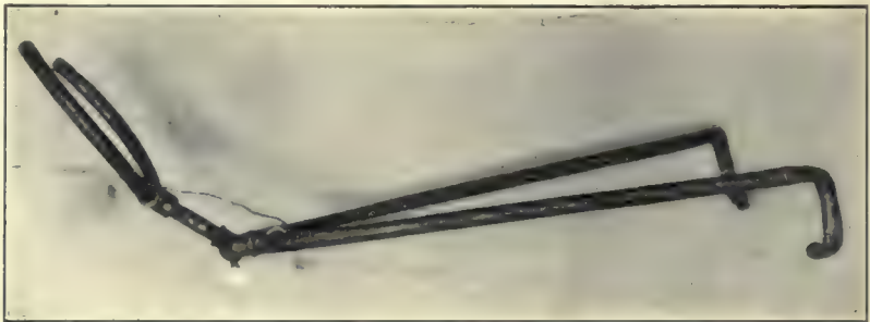
FIG. 93.—Author's Modification of Frazier's Head-rest; Side View. Made of ordinary gas-piping. The head portion is made movable in two directions by inserting two elbows, the joints of which are made tight enough by screws to hold the head in any position. It can be moved up and down, or rotated round the vertical axis.
