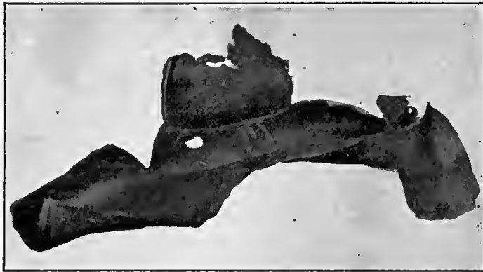
FIG. 203.—Leaden Vessel Filled with Water and Sealed; Showing Explosive Effect Produced by Small-Calibre Bullet Passing through the Water at high Velocity. ("Wounds in War," Stevenson.)
