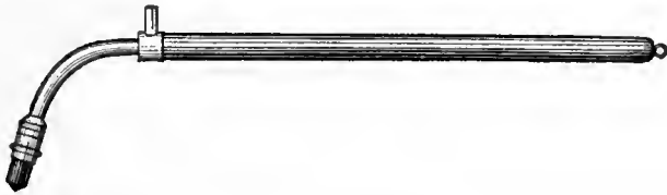
FIG. 50.—Electrode with Carbon Point, for single spark. (C. W. Allen: "Radiotherapy and Phototherapy.")
