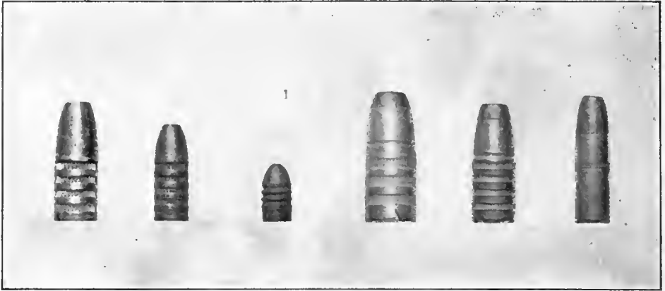
FIG. 199.—Hunting-Rifle Bullets, .22 to .38 Calibre. Three to left, unjacketed; three to right, soft-nosed.
