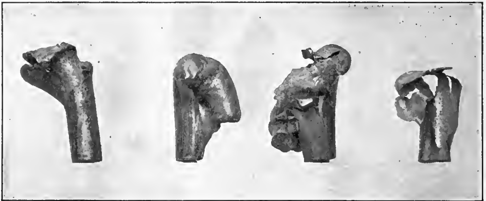
FIG. 201.—30-Calibre Jacketed Bullets Deformed by Ricochet.
