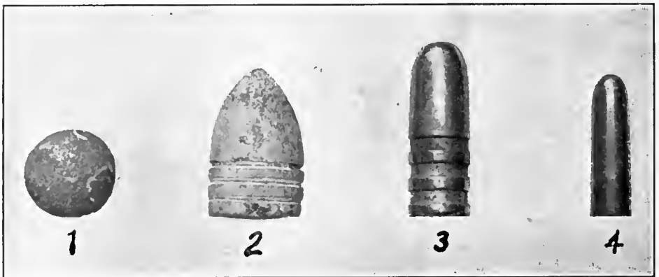
FIG. 200.—Evolution of the Bullet. 1, Old round musket-ball; 2, Minié bullet; 3, .45-calibre Springfield; 4, .30-calibre jacketed Springfield, model 1905. All of natural size.
