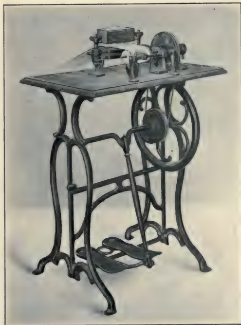
FIG. 364.—Plaster-of-Paris Attachment to Foot Machine.
