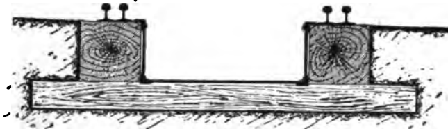
FIG. 39.—PROPOSED DESIGN FOR SHALLOW MAIN TRACK PIT.
