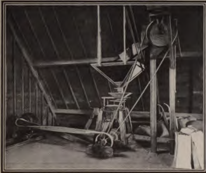
A MOTOR-DRIVEN GRIST MILL IN A BARN, (Saving the expense of buying feed.)
