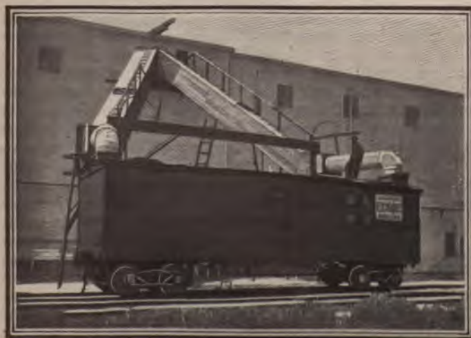
EXPERIMENTAL PRECOOLING PLANT, USED AT LOS ANGELES, CAL., TO LOWER THE TEMPERATURE OF ORANGES BEFORE SHIPMENT.
