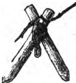
METHOD OF LASHING A PAIR OF SHEERS.
