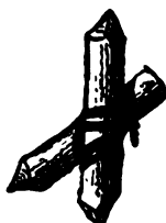
METHOD OF LASHING A DIAGONAL BRACE TO AN UPRIGHT SPAR.
