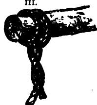
METHOD OF LASHING A PAIR OF SHEERS.
