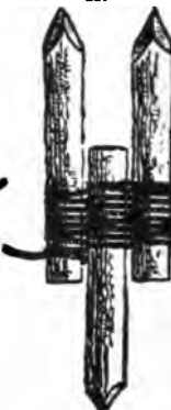
METHOD OF LASHING A TRIPOD TRESTLE.
