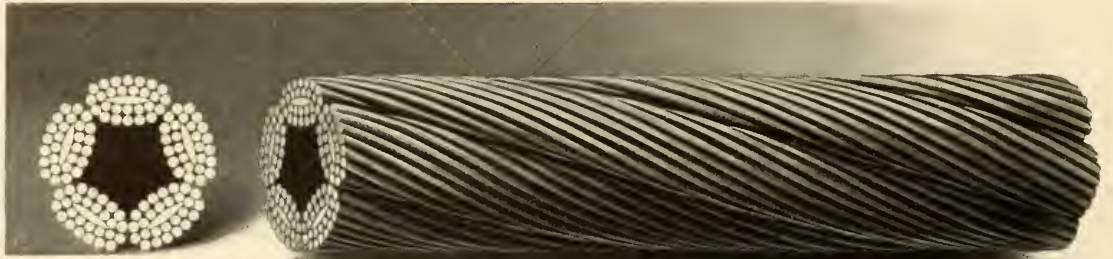
Type A—5 Strands 28 Wires—1 Hemp Core
