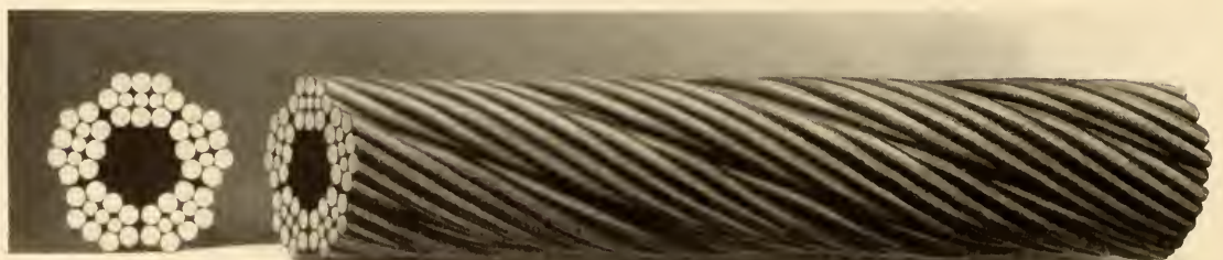
Type E—5 Strands 11 Wires—1 Hemp Core
