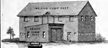
COMPARATIVE SIZE OF STABLE FOR 100 TEAMS, 50 WAGONS, FEED AND HARNESS AND OF GARAGE FOR 15 MOTOR TRUCKS TO DO AN EQUIVALENT AMOUNT OF WORK - FUEL STORED UNDERGROUND
