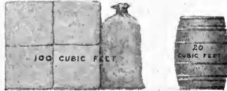
BALED HAY AND OATS GASOLINE COMPARATIVE SPACE REQUIRED FOR STORAGE OF TEAM FEED AND OF GASOLINE FOR ONE MONTH
