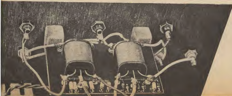
Section of UNIT "B" panel (viewed from rear) showing integrator switch relay assembly
