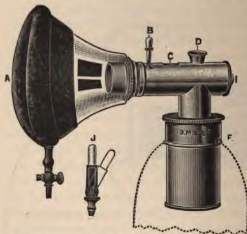
FIG. 50. "Ideal Inhaler"* (Vernon Knowles). A, mask with pneumatic rim; B, lever controlling air inlet; C, air inlet; D, supply aperture fitted with worm to fix capsule crusher, which is shown at J; F, connexion to rubber bag.
