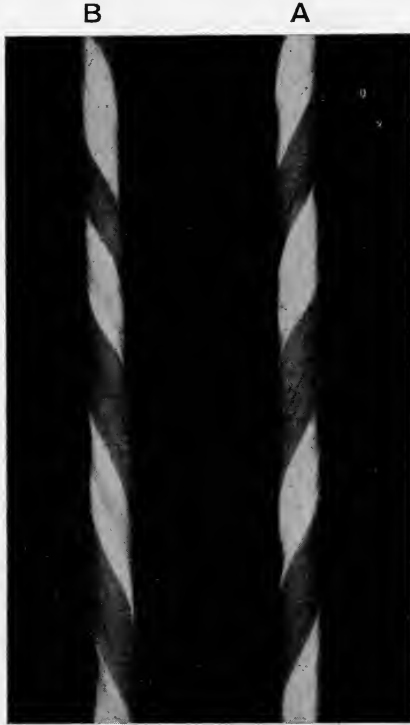
FIG. 14.—A, openband (right twist); B, crossband (left twist).
