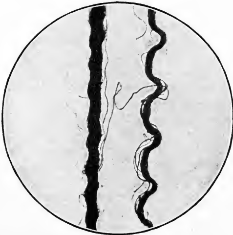
FIG. 50.—Micrograph of thread (a) and pick (b) from cashmere twill cloth.
