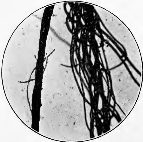
FIG. 9b.—Union yarn. Micrograph of cotton (a) and wool (b) yarns twisted together.
