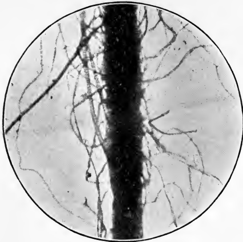
FIG. 9a.—Union yarn. Micrograph of cotton and wool mixture yarn.
