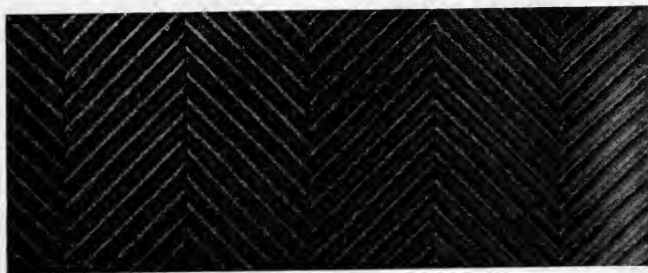
FIG. 16.—Illustrating the influence of direction of twist on twill.
