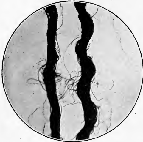
FIG. 48.—Micrograph of thread (a) and pick (b) from corkscrew cloth.
