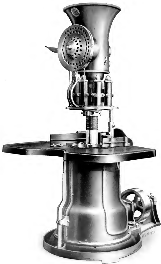
AUTOMATIC POWER CROWN MACHINE INVENTED BY WILLIAM PAINTER. THE CROWNING CAPACITY OF THIS MACHINE IS FROM NINETY TO ONE HUNDRED BOTTLES PER MINUTE. OWING TO ITS ENORMOUS EFFICIENCY IT IS KNOWN BY THE BOTTLING TRADE AS THE "JUMBO."
