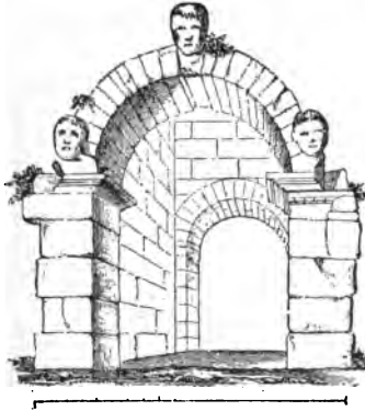
GATE AT VOLATERRÆ, SHOWING THE PRINCIPLE OF THE ARCH.
