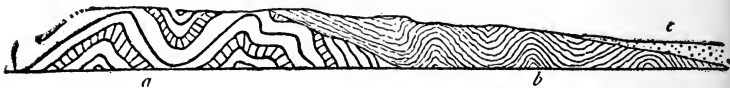
Fig. 20—Diagrammatic section of the Laurentian Rocks in Lower Canada. a Lower Laurentian; b Upper Laurentian, resting unconformably upon the lower series; c Cambrian strata (Potsdam Sandstone), resting unconformably on the Upper Laurentian.
