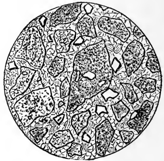
Fig. 6.—Microscopic section of a calcareous breccia in the Lower Silurian (Coniston Limestone) of Shap Wells, Westmoreland. The fragments are all of small size, and consist of angular pieces of transparent quartz, volcanic ashes, and limestone embedded in a matrix of crystalline limestone. (Original.)
