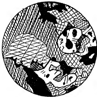
Fig. 21.—Section of Lower Laurentian Limestone from Hull, Ottawa; enlarged five diameters. The rock is very highly crystalline, and contains mica and other minerals. The irregular black masses in it are graphite. (Original.)
