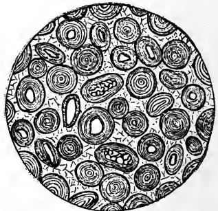
Fig. 13.—Slice of oolitic limestone from the Jurassic series (Coral Rag) of Weymouth; magnified. (Original.)
