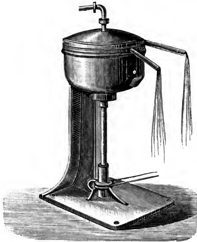
FIG. 41. The De Laval Separator. (Elevation.)
