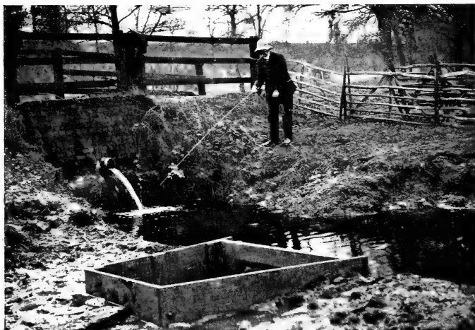
Observation Tank in the bank of a controlled stream.
