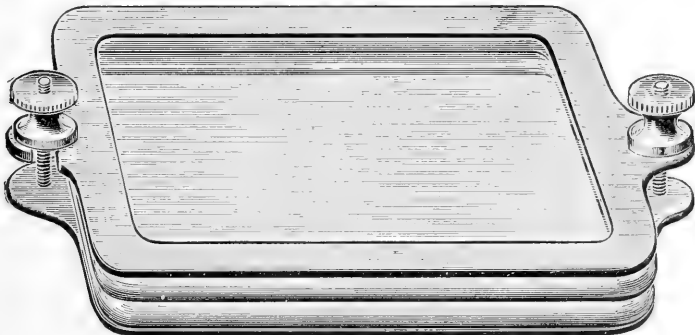
FIG. 71.—Compressor Used by the Government Bureaus for Meat Inspection.
