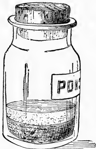
FIG. 241. Insect killing-bottle; cyanide of potassium at bottom, covered with plaster of Paris.
