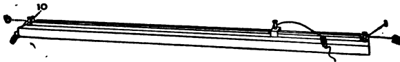
Fig. 5. The rheocord. A metre rule is screwed to the lid of a shallow box of oak. At each end is a binding post. To the post marked 0 is fastened one end of an unbroken German silver wire (No. 30) ten metres in length. This wire passes over the metre stick to post 1, and thence into the box, where the remaining nine metres go to and fro between two rows of pegs at the ends of the under side of the cover of the box. The end of the 10 metre wire is brought out of the box and fastened to post 10.
