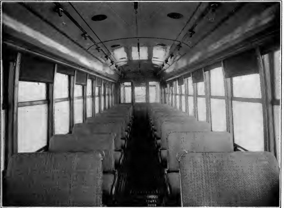
INTERIOR OF PLAIN ARCH ROOF CAR. SPACE BETWEEN CEILING AND ROOF UTILIZED FOR VACUUM VENTILATING SYSTEM. THIS TYPE OF ROOF PERMITS THE WINDOW OPENINGS TO BE 4\frac{1}{2} INCHES HIGHER THAN STANDARD.
