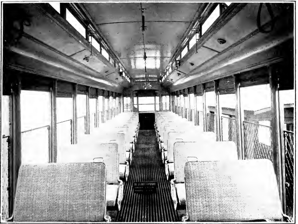
INTERIOR OF CONVERTIBLE CAR ARRANGED FOR SUMMER SERVICE. SEATING CAPACITY, 45.
