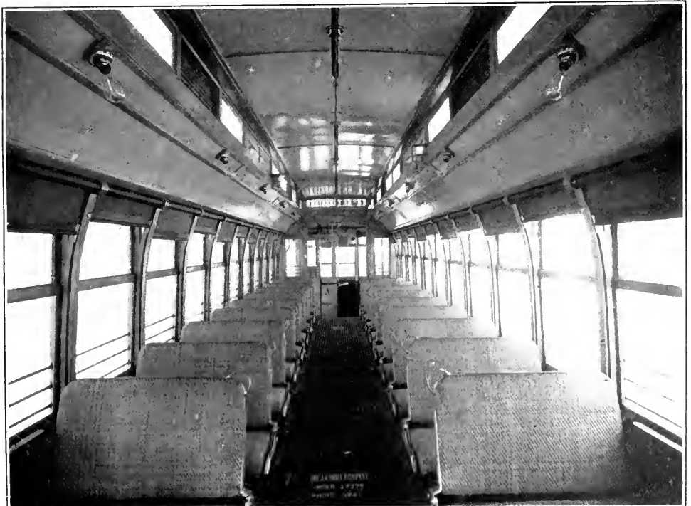
INTERIOR OF SEMI-CONVERTIBLE CAR. BOTH UPPER AND LOWER SASHES RAISE INTO ROOF POCKETS.
