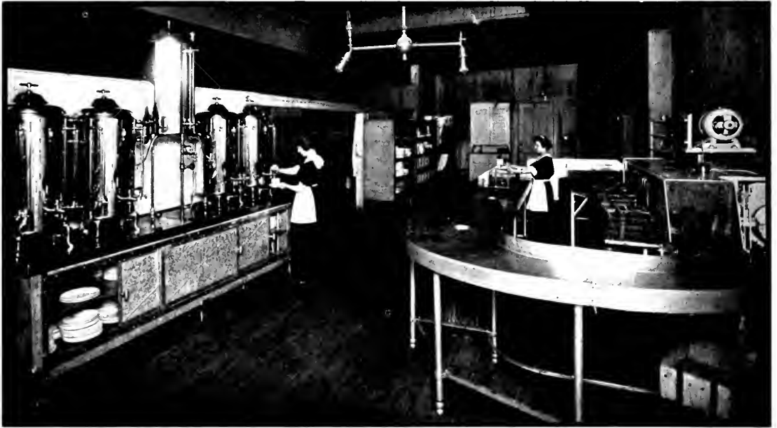
Dish Room—The Niagara Dish Washer at Right Handles 1000 Dishes an Hour—Tea and Coffee Urns at Left
