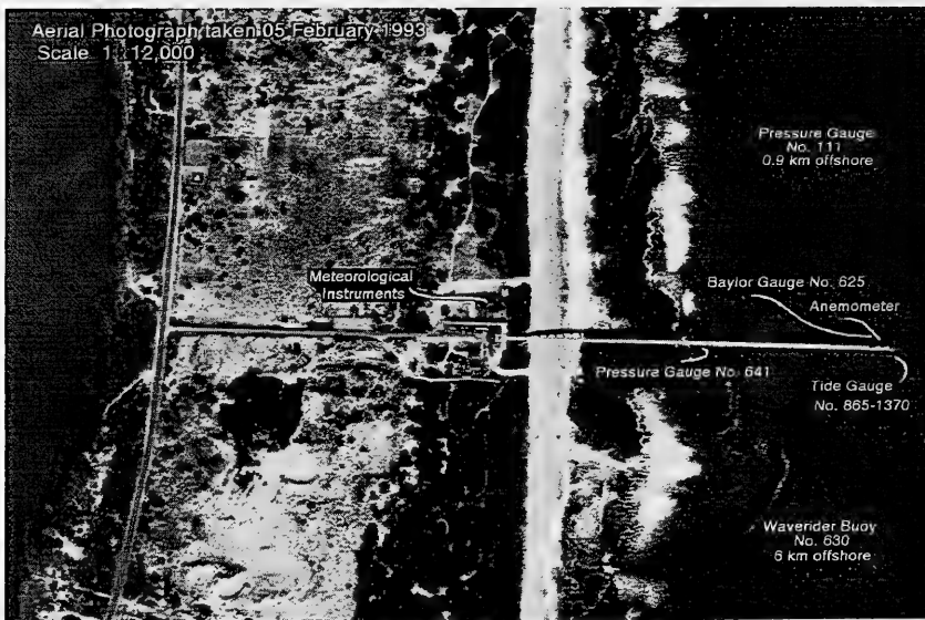
Figure 2 . FRF gauge locations
