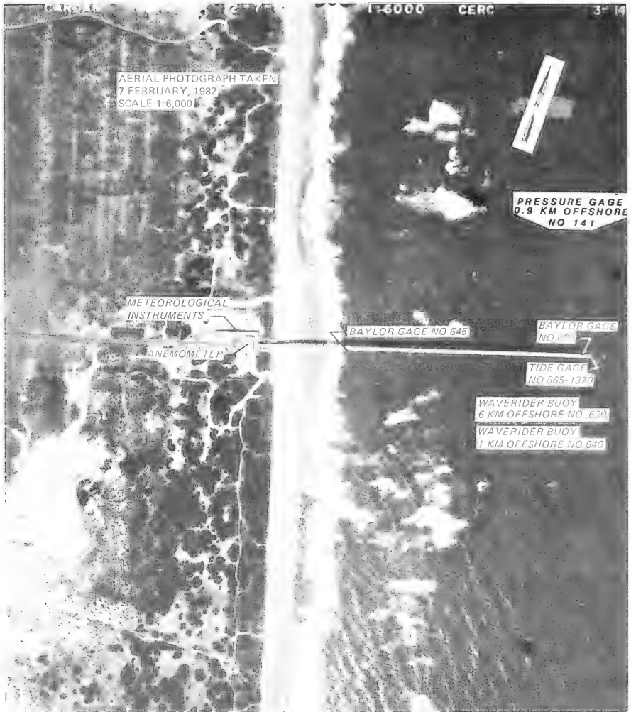
Figure 2. FRF gage locations
