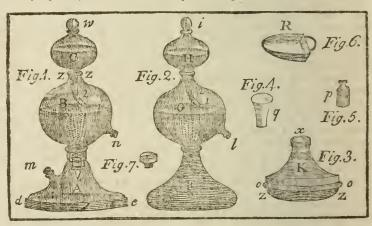
HE following description of an apparatus for impregnating water with fixed air is extracted from an account, publish-
