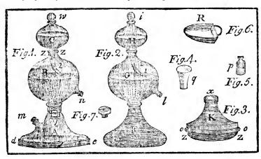
HE following description of an apparatus for impregnating water with fixed air is extracted from an account, published by the ingenious Mr. Magellan, of his improved method of performing that operation. It can scarcely be necessary to inform our read-
