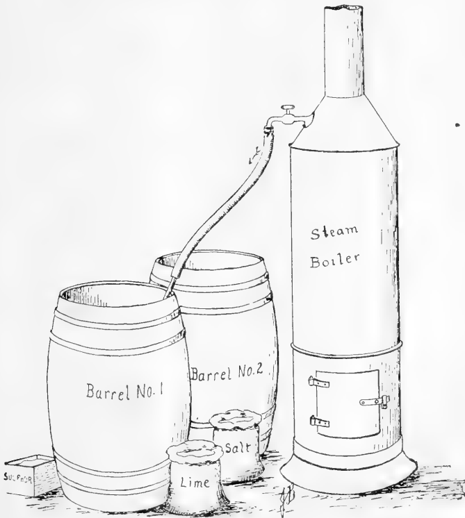
Fig. 9 a W. W. Hilborn's appliance for making the lime-sulphur-salt mixture.
