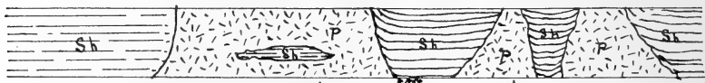
Fig. 4 Section of Green street dike along excavation made by electric light company, November 24, 1905. Sh = shale P = peridotite
