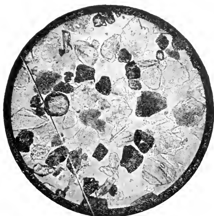
FIG. 5.—Micro-photograph of fine sand soil showing the irregular shape of the particles and their difference in mineral composition. The mineral plant foods are contained in these particles of mineral
