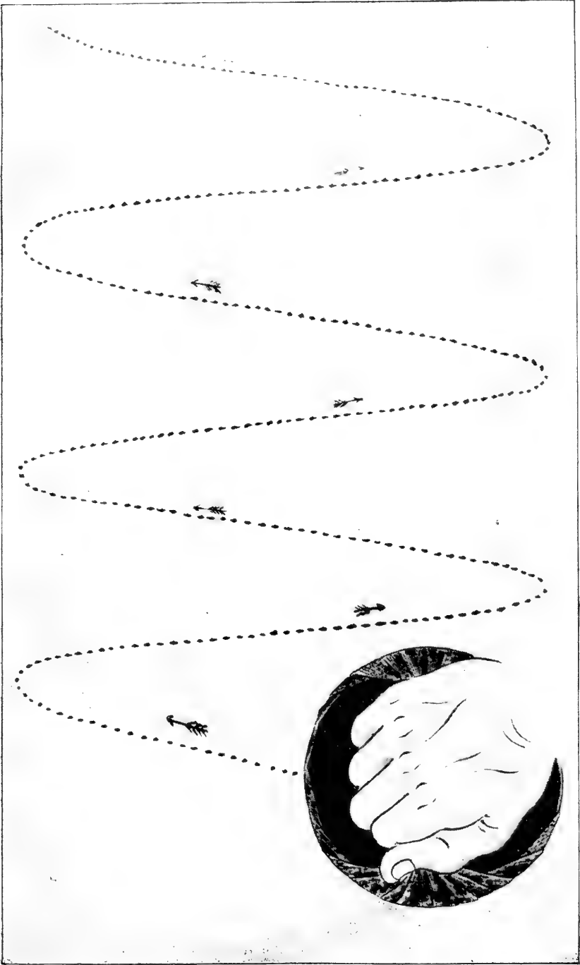
METHOD OF USING BAREN. (From a drawing in the U. S. National Museum by a Japanese artist.)
