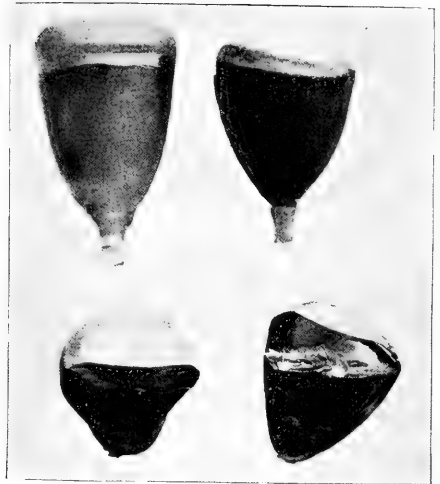
2. "BOULES" OF ARTIFICIAL CORUNDUM.
