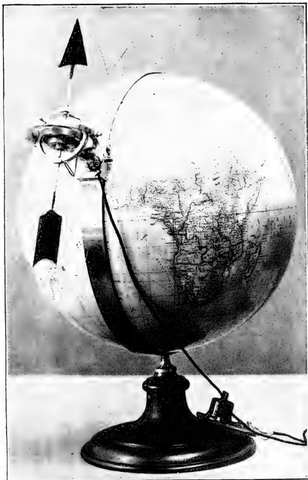
DEMONSTRATION MODEL OF GYROSTATIC COMPASS.
