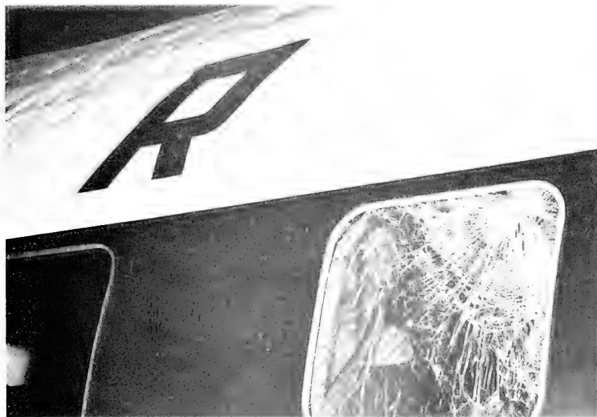
2. Hail damage to Convair aircraft parked at Grand Island Airport, June 27, 1959. (Frontier Airlines photograph.)
