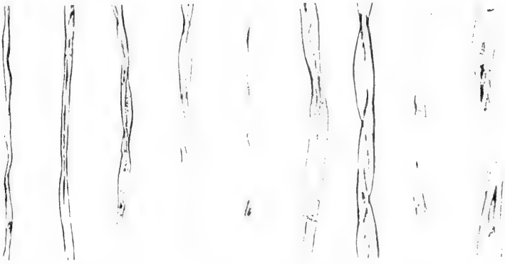
1. Composite photomicrograph of longitudinal views of mature fibers showing different degrees of fineness over a wide range as found in American upland cotton. Magnification in all cases X 165.
