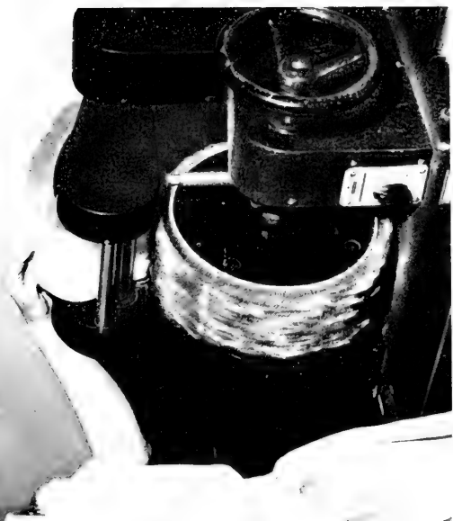
2. Technician blending a sample of ginned lint using the Gaus-Larrison mechanical cotton fiber blender. Owing to the great variations existing in the distribution and proportions of cotton fiber types throughout a sample, the determination of most fiber properties requires a preblending of the cotton in order to give representative and reliable test specimens.
