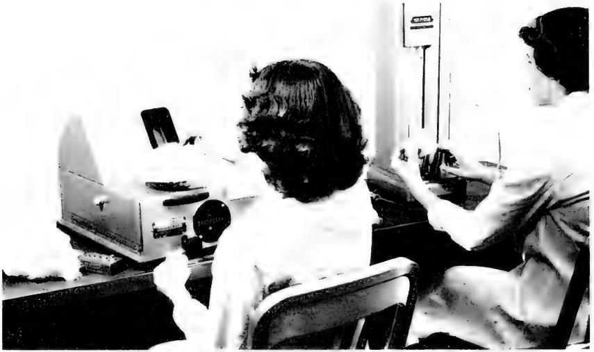
1. Technicians using the Smith-Sheffield Micronaire instrument to evaluate fiber fineness and maturity in combination as possessed by cotton lint. The Micronaire scale values observed represent averages for the respective test specimens.
