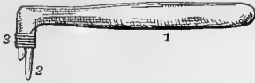
FIG. 28.—The Weubaja. (1) The horn. (2.) The iron (side view). (3) Sinew tied around the iron.
