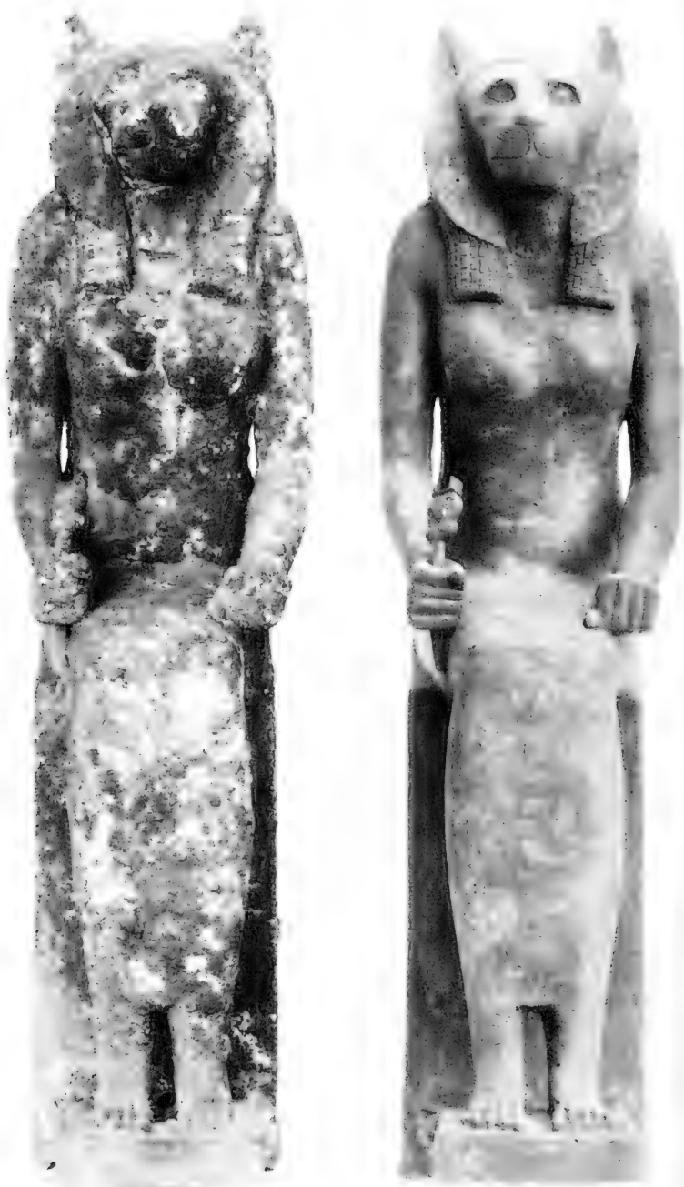
EGYPTIAN BRONZE STATUE OF THE LION-HEADED GODDESS SEKHMET. BEFORE AND AFTER ELECTROCHEMICAL TREATMENT.
