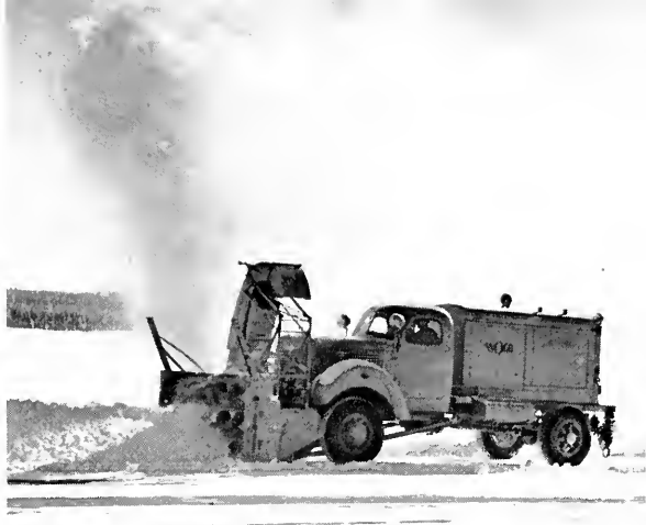
The Highway Division's rotary snow plow is shown clearing an airport runway
