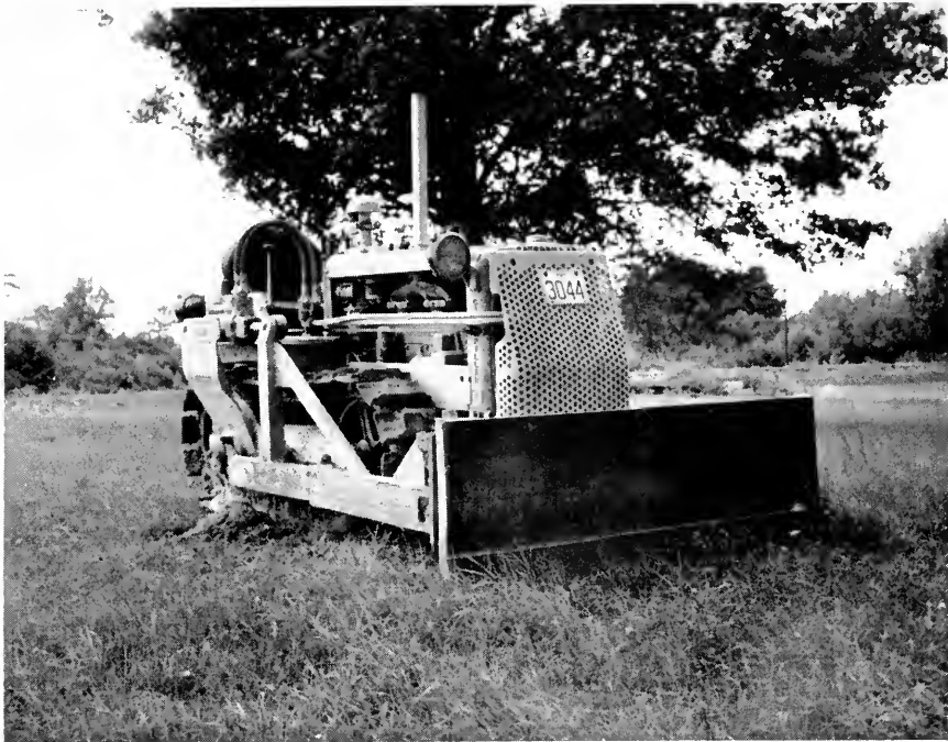
The Water Department's new 5-ton bull-dozer is used both for filling ditches and snow removal.
