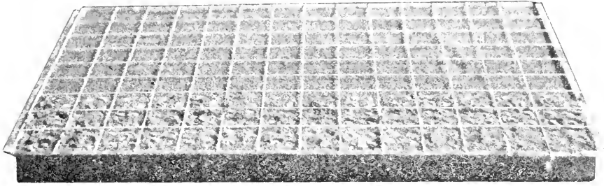
FIG. 4.—Galvanized iron germinator, described on p. 9. Small notches are cut in the rim at intervals of 1\frac{1}{4} inches to carry the string or wire which divides the germinating surface into 1\frac{1}{4} inch squares. This figure shows four rows of kernels in place.
