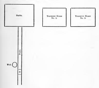
This well furnished all the water for both houses. Drain obstructed completely at the point marked (a), as was ascertained by digging it out at time when patients were sick. As the soil was firm and solid the well must have received drainage from the stable, privy, etc. My first patient came from Pittston, sick, into tenement No. 2.
