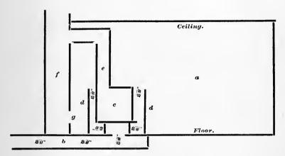
a represents the school-room; b, the fresh air box; c, the stove; d, d, the sheet iron jacket around the stove, enclosing its sides except the door; e, the stove pipe; f, the chimney, which serves as a smoke flue and at the same time as a ventilation flue, by leaving an opening near the floor level at g.
