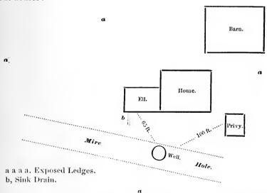
It will be seen that the arrangements were such that the westerly breezes might waft the poisonous vapors from the privy to the house, and that the well might have the benefit of the soakage from both the privy and the sink spout. Undoubtedly the typhoid fever germs in the discharges of the former patient found their way from privy or slop hole at back door, or both, to the well and were the cause of the father's illness and death.
