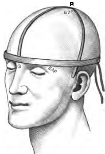
FIG. 3.—WILSON'S CYRTOMETER ( in situ ). G, glabella; E A P, external angular process; R, fissure of Rolando, its position and direction marked by the lateral strip of metal.
