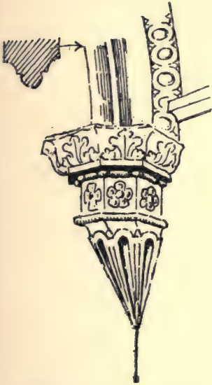
BARLBOROUGH HALL: CORBEL IN PORCH.
