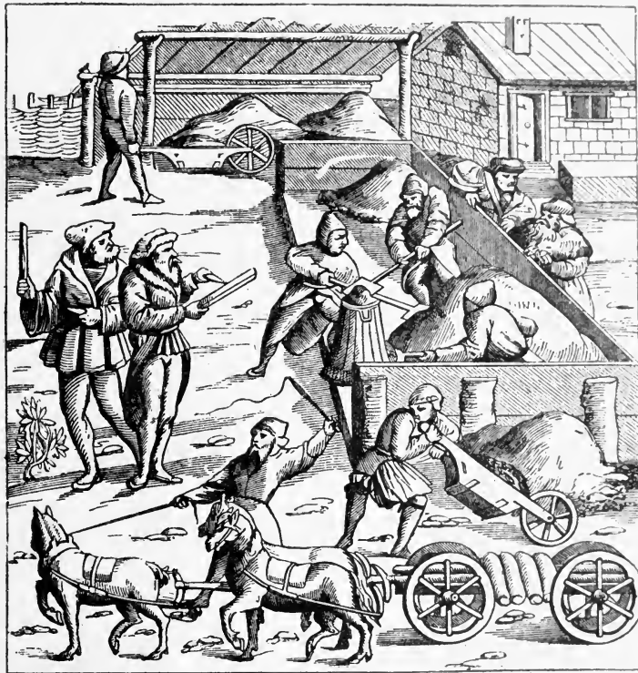
SORTING THE ORE: THE TWO MASTERS ON THE LEFT ARE TRYING THE "STREAK" ON THE TOUCHSTONE.
