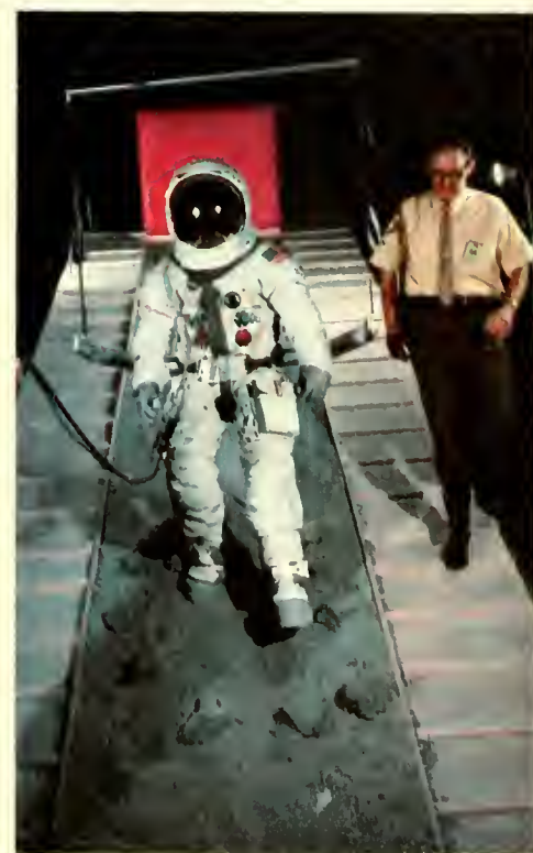
Partly suspended, Apollo 14 commander Shepard familiarizes himself with the one-sixth of normal gravity on the Moon by using a low-gravity simulator during training
