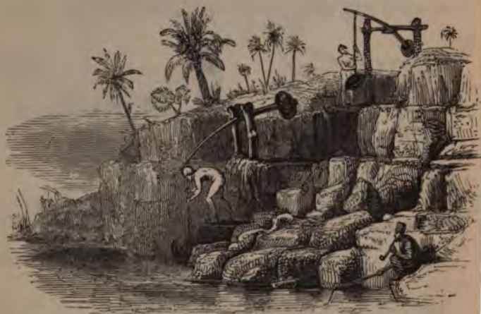
a. Modern shadóf , or pole and bucket, used for raising water, in Upper and Lower Egypt.
